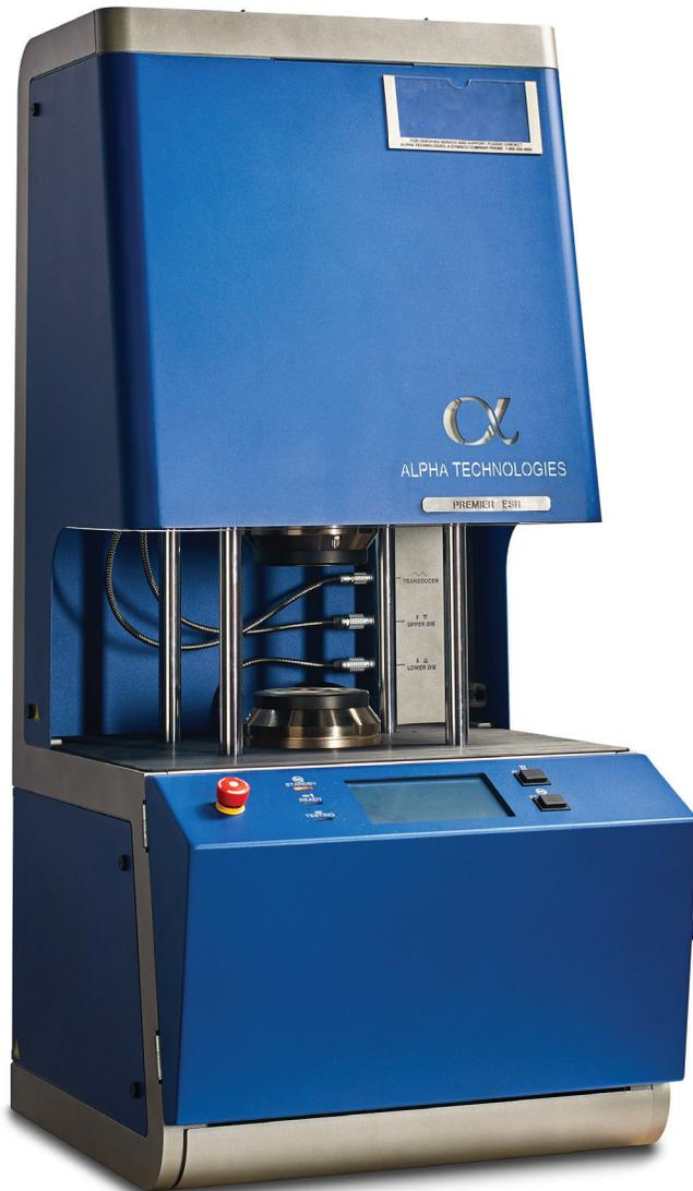
▶ The ESR is an instrument for Quality Control and Research & Development. Data provided includes: viscosity, gel time, cure time, reaction rate, final modulus and glass transition temperature. The ESR's advanced temperature control system allows measurements under isothermal and nonisothermal conditions.
